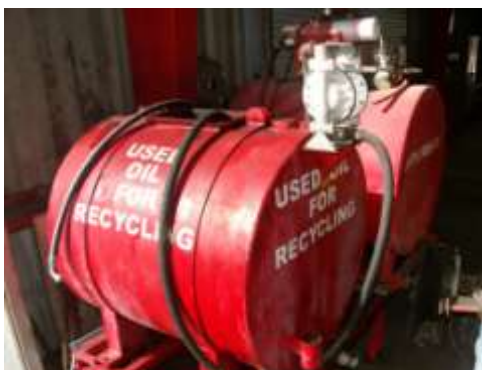
Ranger Construction Industries Photo: Used oil collection tank and antifreeze recycling machine.
