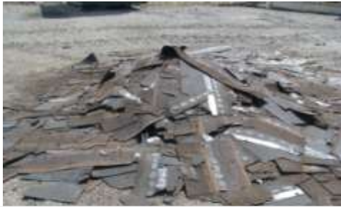
APAC KS-MO Photo: Tear-off shingles pile prior to processing.
