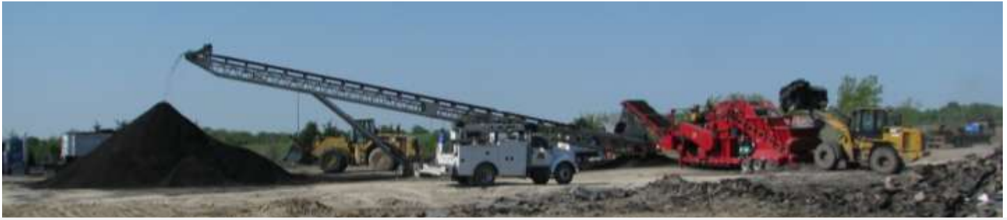
APAC KS-MO Photo: Processing of tear-off shingles for use in asphalt mix.
