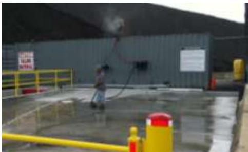
Lane Construction Corporation Photo: Water is recycled at Occoquan, VA shop where the recycling equipment washing station keeps the fleet lean and clean while being green. Zero discharge is accomplished with an evaporation technique.
